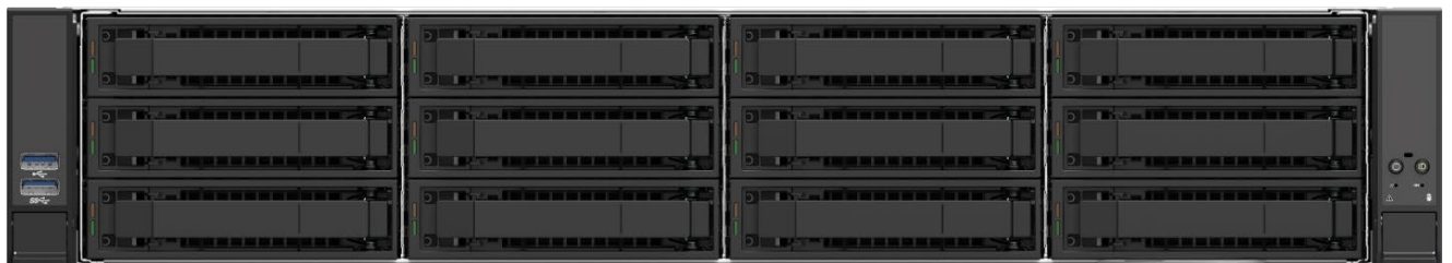
Figure 11. 12 x 3.5" Front Drive Bay Configuration – M50FCP2UR312
