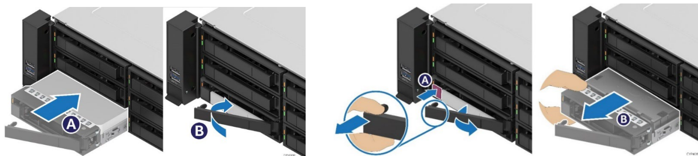
Figure 64. 3.5" Drive Insertion / Extraction
