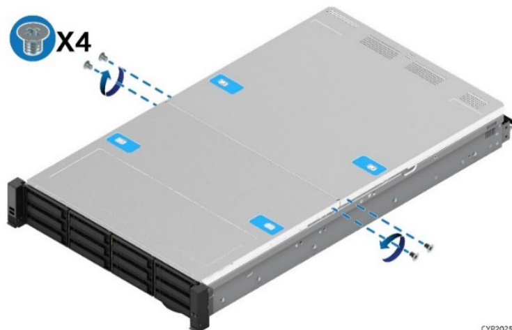
Figure 23. Top System Cover Panels Shipping Screws
