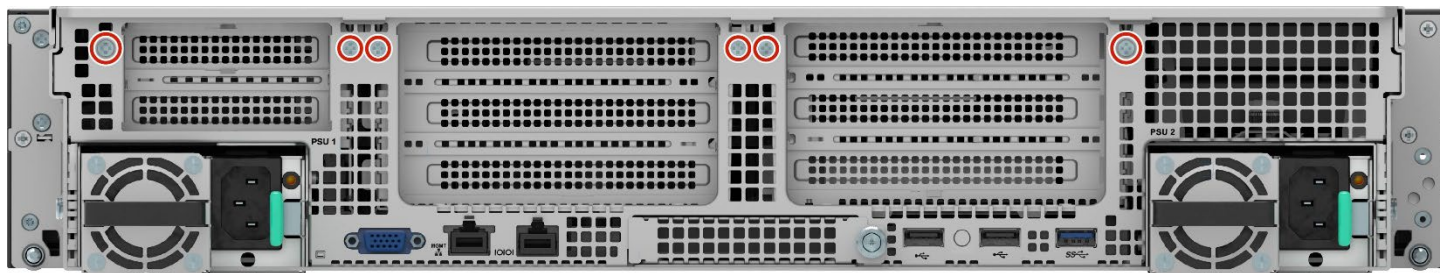
Figure 27. Rear Panel Shipping Screw Holes
