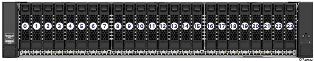
Figure 72. 24 x 2.5" Front Bay Drive Configuration – M50FCP2UR208 with accessory options
