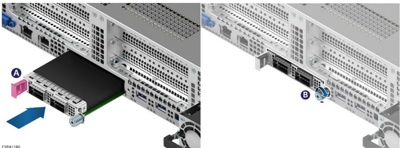
Figure 58. OCP* Adapter with Pull Tab Installation
