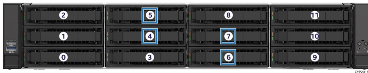
Figure 77. 12 x 3.5" Front Bay Drive Configuration – M50FCP2UR312
