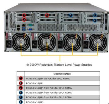
4x 3000W Redundant Titanium Level Power Supplies
