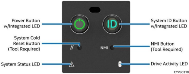
Front Control Panel
