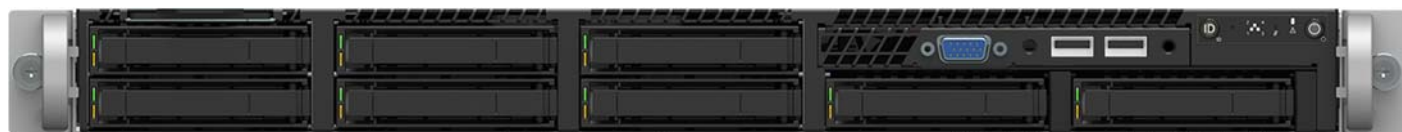
Figure 11. 2.5" Drive Bay – 8 Drive Configuration (Model R1208WFxxx)
