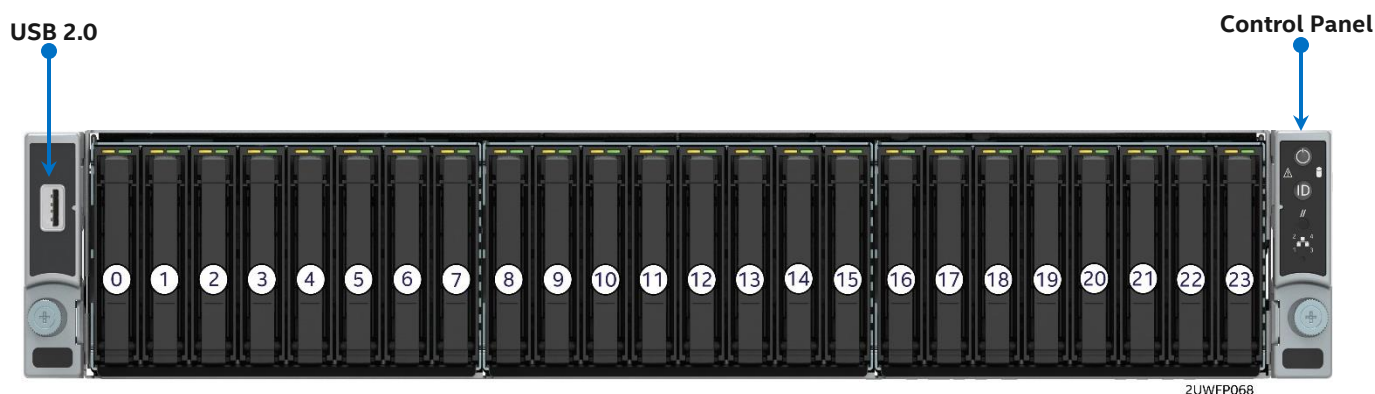
Figure 42. 2.5" front mount drive bay, 24-drive (R2224WFXXX) configuration
