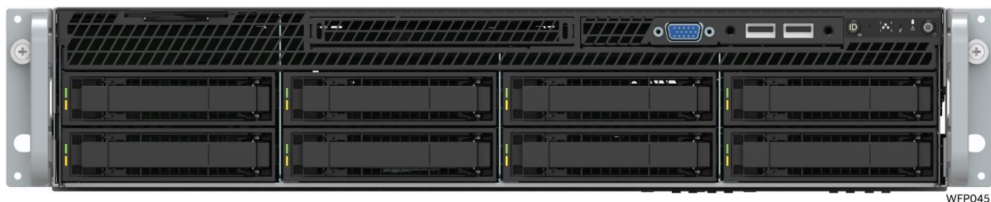
Figure 11. 3.5" x 8 front drive bay configuration – R2308WFxxxx
