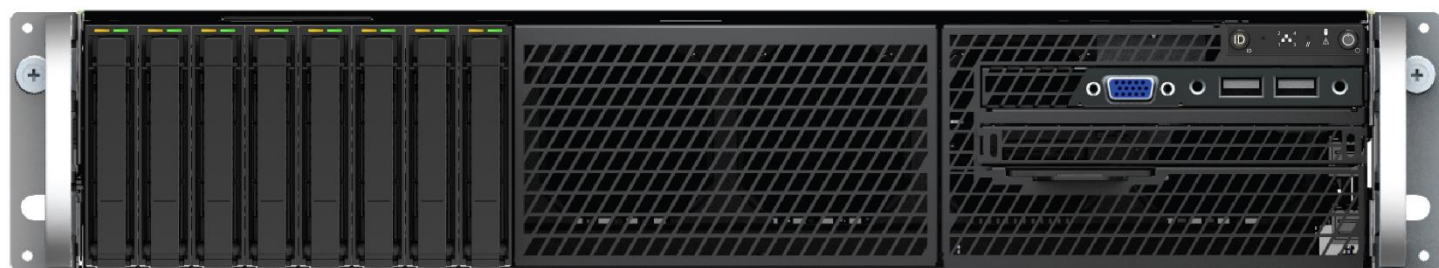
Figure 13. 2.5" x 8 front drive bay configuration – R2208WFxxxx
