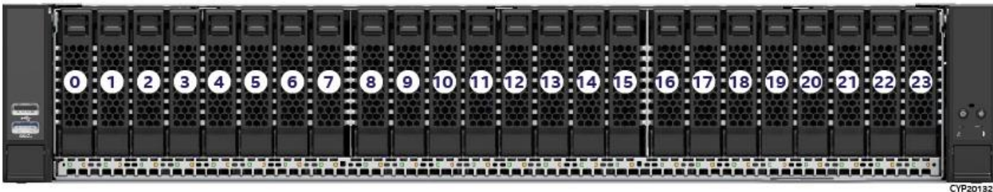
Figure 66. 24 x 2.5" Front Bay Drive Configuration (based on M50CYP2UR208)
