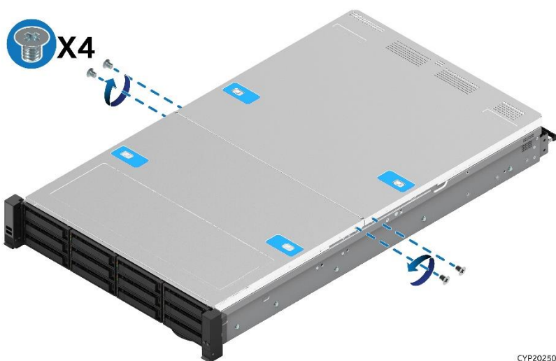
Figure 19. Top System Cover Panels Shipping Screws
