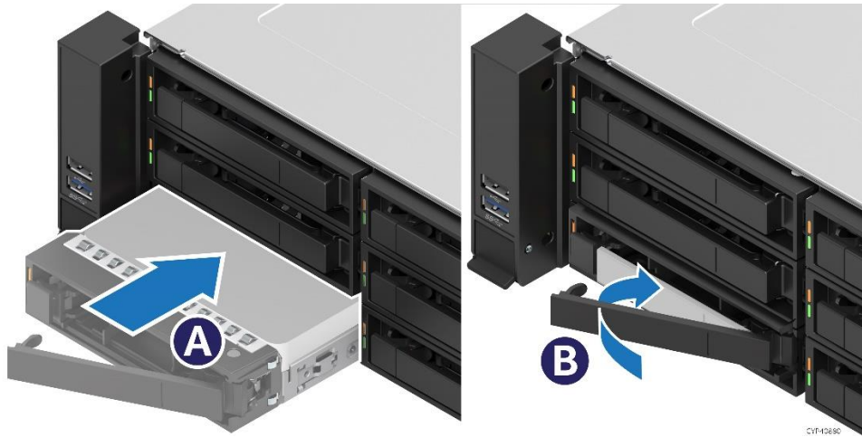
Figure 79. Drive Insertion into 3.5" Drive Bay
