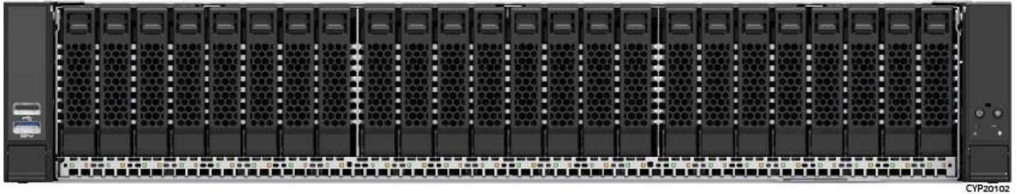
Figure 8. 24 x 2.5" Front Drive Bay Configuration (based on M50CYP2UR208)
