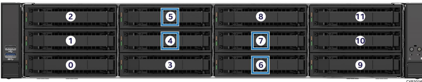
Figure 67. 12 x 3.5" Front Bay Drive Configuration – M50CYP2UR312
