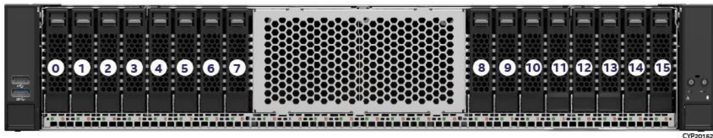
Figure 65. 16 x 2.5" Front Bay Drive Configuration (based on M50CYP2UR208)
