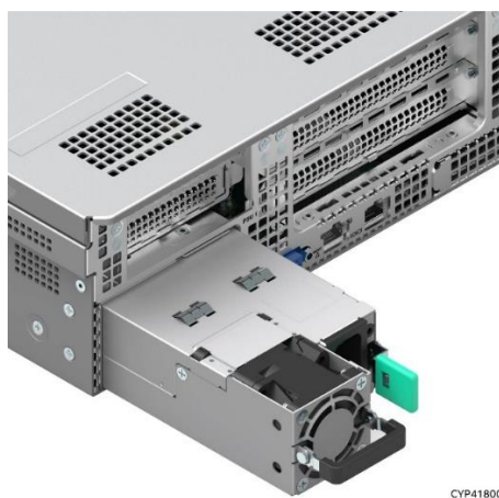
Figure 34. Power Supply Module Partially Out of Chassis
